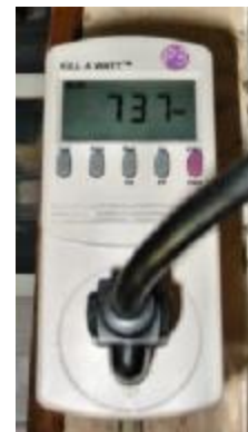
DeLonghi electric space heater, 1500 watts. It has three settings that are supposed to use 1500, 900 and 600 watts. On high, it used around 1520 watts and on medium and low it used around 737 watts.
