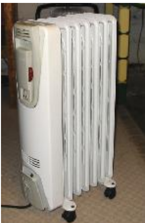
DeLonghi electric space heater, 1500 watts. It has three settings that are supposed to use 1500, 900 and 600 watts. On high, it used around 1520 watts and on medium and low it used around 737 watts.
