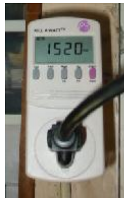
DeLonghi electric space heater, 1500 watts. It has three settings that are supposed to use 1500, 900 and 600 watts. On high, it used around 1520 watts and on medium and low it used around 737 watts.
