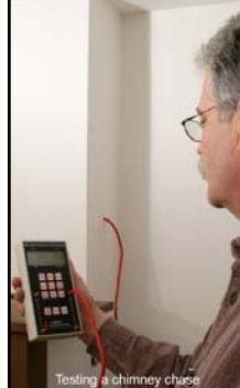
Testing a chimney chase
